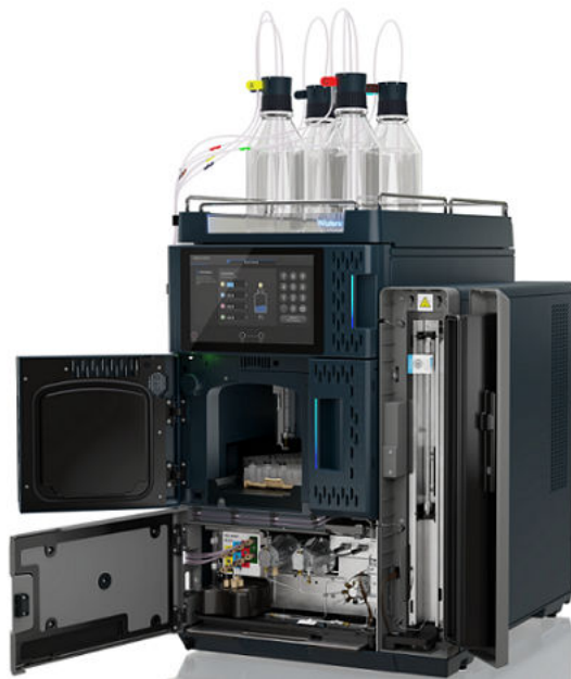
Figure 6–3: Connected solvent bottles
