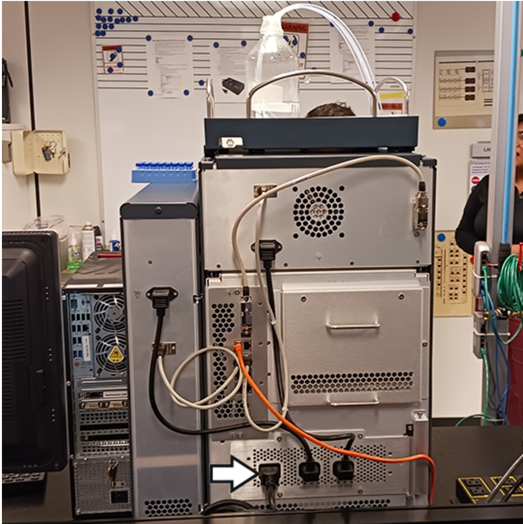
Figure 4–2: Connecting power cable
