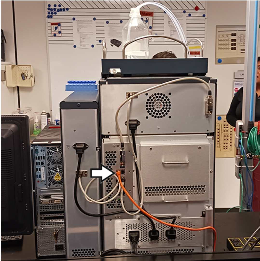
Figure 4–1: Connecting network cable
