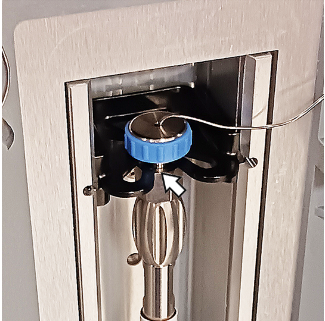
Figure 4–4: Column seated in column clip
