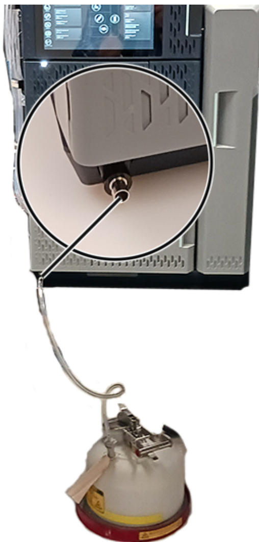
Figure 4–3: Connecting the system to a waste container
