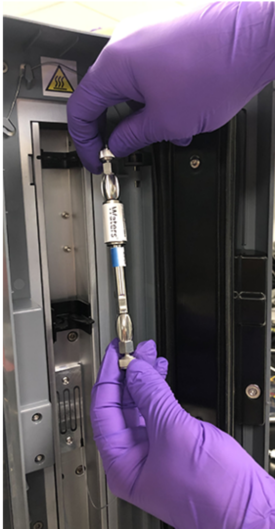
Figure 8–102: Installing the replacement column
